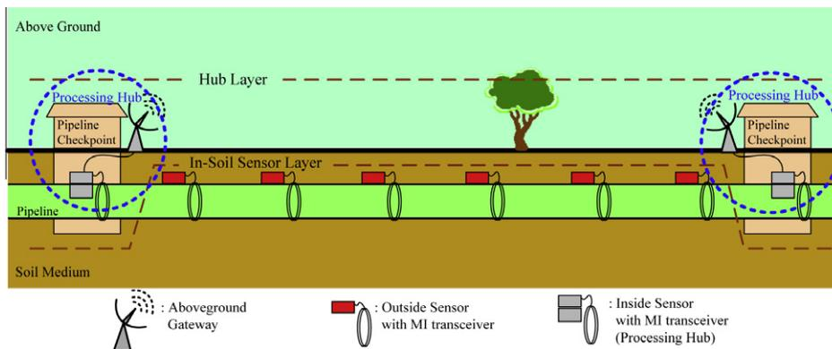
Fig. 1. System architecture of MISE-PIPE.
