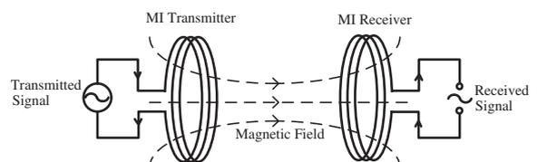
Fig. 2. MI-based wireless communications.
