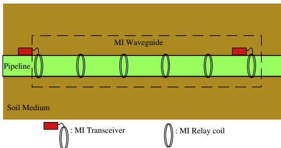
Fig. 3. MI waveguide structure in MISE-PIPE.
