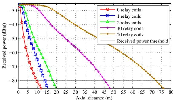
Fig. 4. Received power of MI waveguides with different numbers of relay coils.
