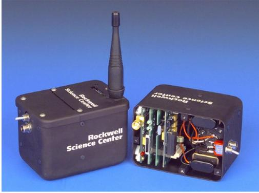
Figure 1: WINS Sensor Node from RSC
