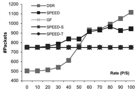
Figure 11. Control packet overhead comparison
