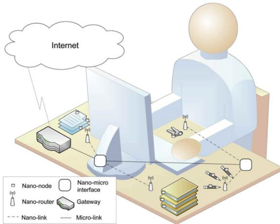
Fig. 11. Network architecture for WSNs in the interconnected office.
