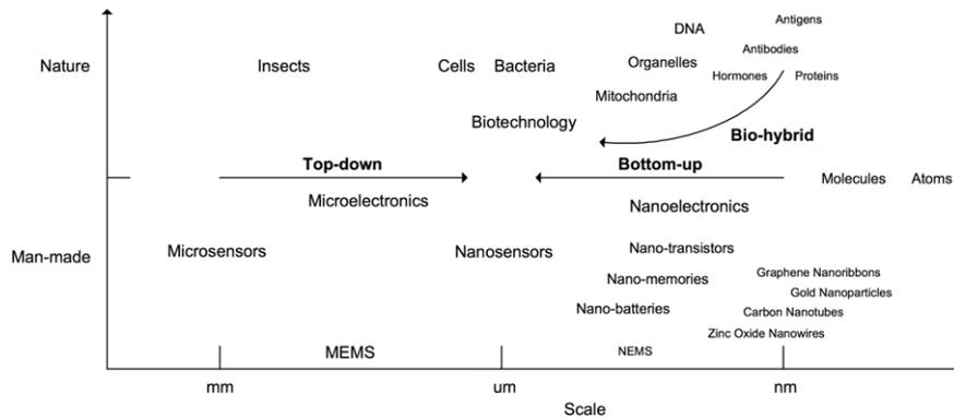
Fig. 7. Approaches for the fabrication and integration of nanosensors.
