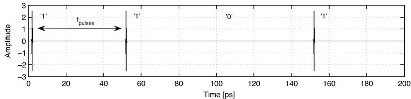
Fig. 15. Pico-pulse-based communications. The time between pulses,  $t_{\text{pulses}} = 50$  ps, is much longer than the pulse length, 0.1 ps in this case.
