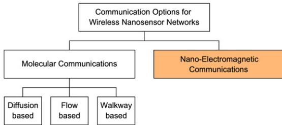
Fig. 1. Communication options for wireless nanosensor networks.
