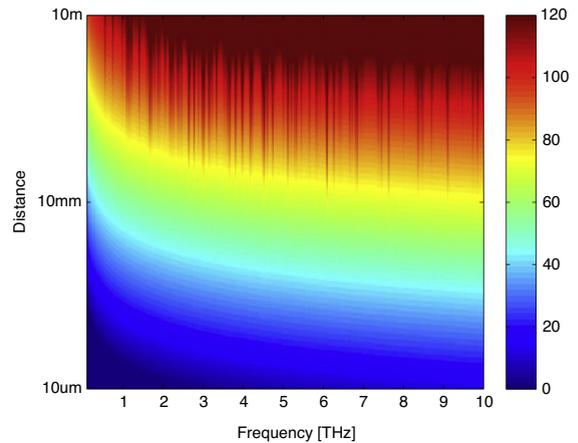
**Fig. 12.** Total path-loss in dB as a function of frequency and distance in a standard medium with 1% of water vapor molecules (the values for path-loss have been truncated at 120 dB to avoid masking relevant transmission windows in the short range).
