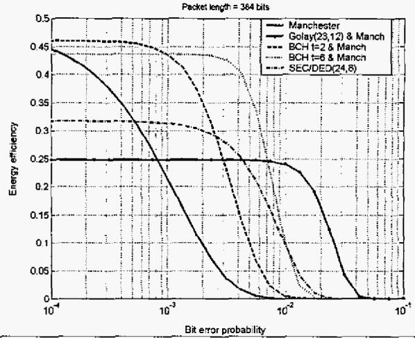
Figure 4. Energy efficiency as a function of bit error probability over a single hop
