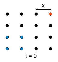
The blue nodes are the source nodes that need to send a packet to the sink (red node). Assume that all immediate horizontal and vertical neighbors of a node are accessible ( $\sqrt{2}*x > R > x$ ). The total time for transmitting a packet is 3 sec.
