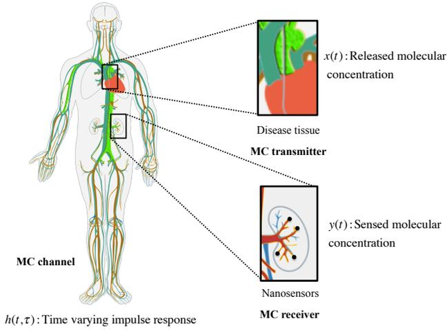
Fig. 2. Scheme of the intra-body molecular communication network for health monitoring and diagnosis.
