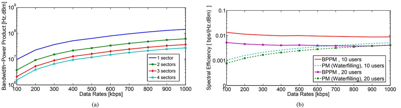
Fig. 9. (a) Beamforming impact on bandwidth-power product utilization for 12 users at different user data rates using 1, 2, 3, and 4 sectors and (b) spectral efficiency of BPPM and PM algorithms for 10 and 20 users at different user data rates.
