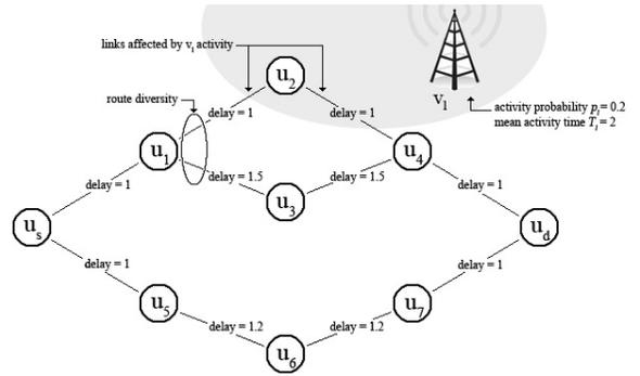
Fig. 2. Metric Accuracy: a metric that neglects the route diversity measures a delay equal to 4.5 for the route  $u_s-u_1-u_2-u_4-u_d$ , although the actual delay for the combined route  $u_s-u_1-(u_2$  when  $v_l$  is not active,  $u_3$  otherwise)- $u_4-u_d$  is 4.2.
