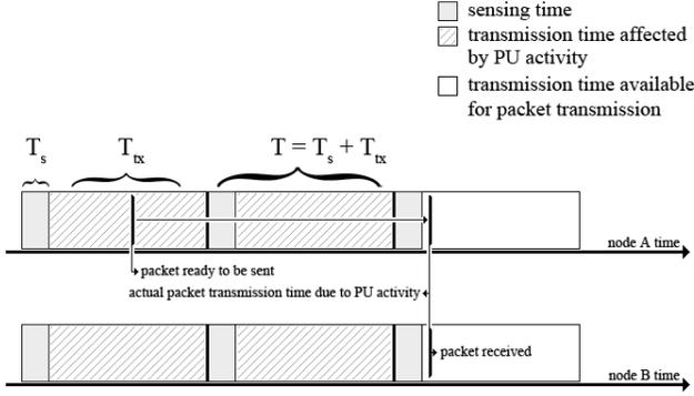
Fig. 3. Link Delay for packet transmission due to the presence of PU activity.
