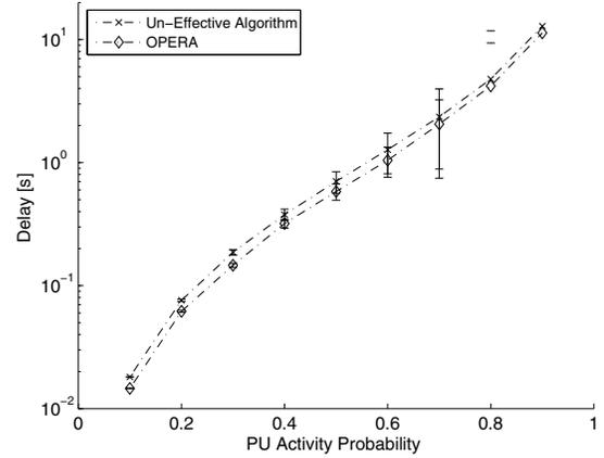
Fig. 8. OPERA accuracy: average delay vs PU activity probability  $p_l$ . Logarithmic scale for axis  $y$ .
