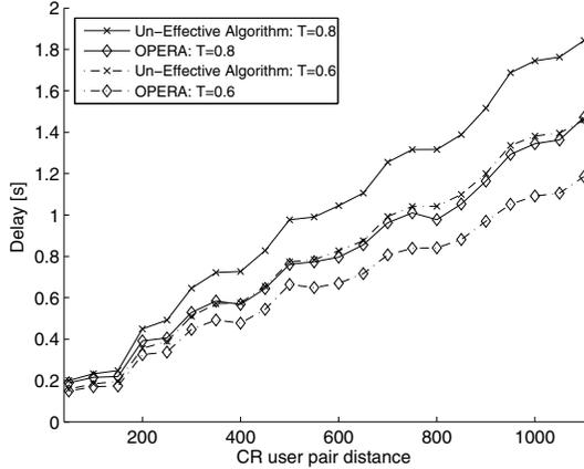
Fig. 11. OPERA accuracy: delay vs CR user pair distance for different values of time period  $T$ .
