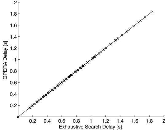
Fig. 7. OPERA optimality: OPERA delay vs Exhaustive Search delay for the topology shown in Fig. 6. For each dot, coordinate  $(x)$  represents the delay computed through exhaustive search, whereas coordinate  $(y)$  represents the delay computed through OPERA expression.
