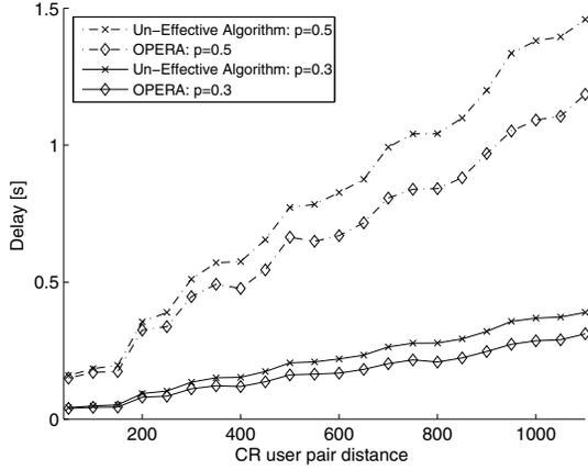
Fig. 9. OPERA accuracy: delay vs CR user pair distance for different values of PU activity probability  $p_l$ .
