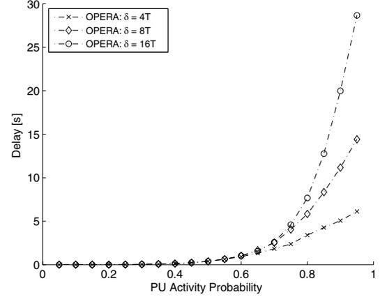
Fig. 12. Mobile networks: OPERA delay vs PU activity probability  $p_l$  for different values of the routing update period  $\delta$  normalized to the time period  $T$ .
