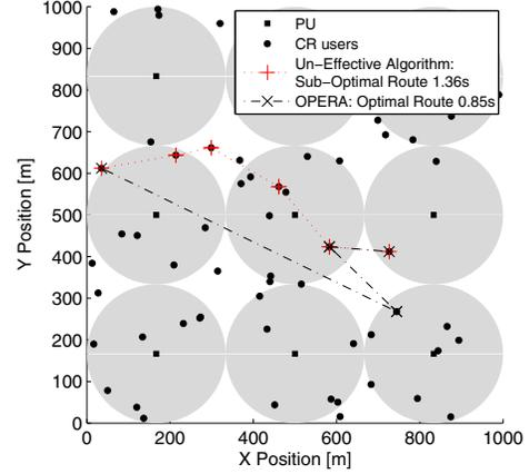
Fig. 6. Considered topology: the figure shows two different routes and the respective delays between the same couple source-destination, the route singled out by OPERA (black line) and the route singled out by the un-effective algorithm.
