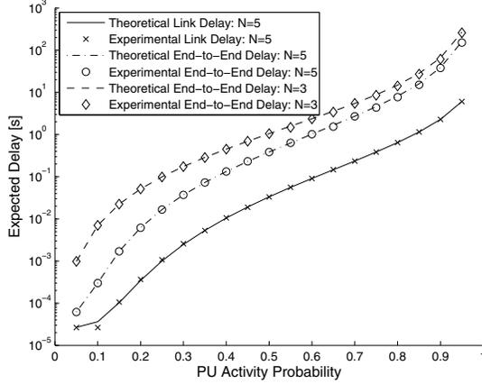
Fig. 5. OPERA validation: theoretical delays vs experimental delays for expressions (9) and (11). Logarithmic scale for axis  $y$ .
