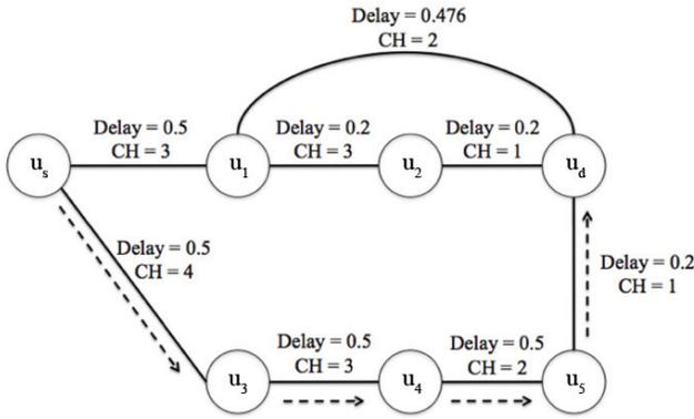
Fig. 1. Metric Optimality: WCETT metric fails in finding the shortest path between  $u_s$  and  $u_d$  whenever  $\beta > 4/9$ , since node  $u_s$  sets  $u_s-u_3-u_4-u_5-u_d$  as the optimal route, although  $u_s-u_1-u_d$  is the actual optimal one.
