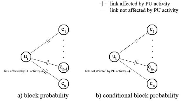
Fig. 4. Difference between Block Probability and Conditional Block Probability.
