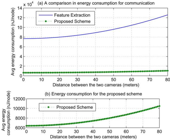
Fig. 10. Average energy consumption for communication per node.
