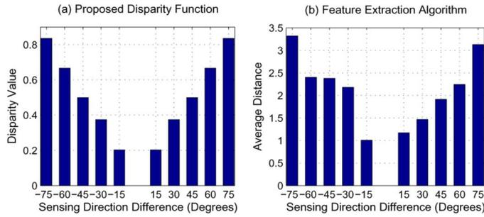
Fig. 9. Proposed disparity function versus feature extraction algorithm.
