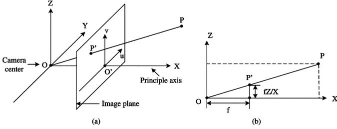
Fig. 2. Camera projection model.
