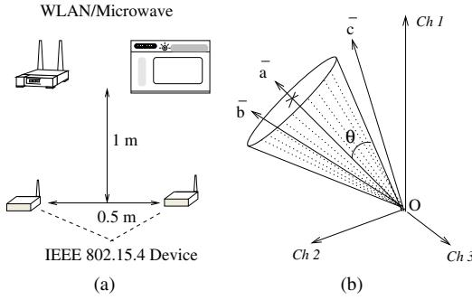
Fig. 1. The experimental setup to measure the WLAN and microwave interference (a) and the allowed conical region for classification of the interferer (b).
