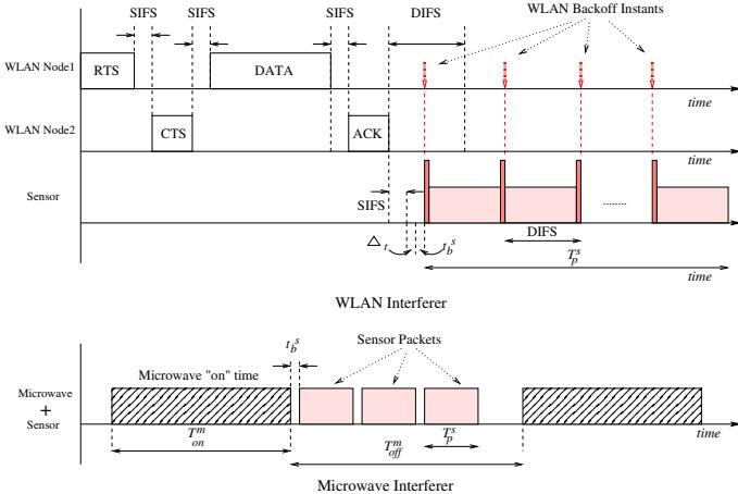
Fig. 3. The sensor transmits whenever the channel is free based on the WLAN traffic or microwave duty cycle.
