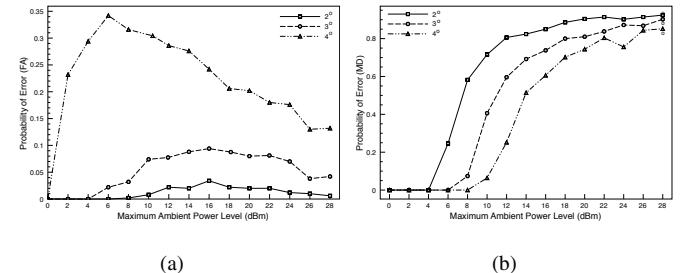
Fig. 4. The probabilities for false alarm (FA) and missed detection (MD) for the spectral signature matching technique are given in (a) and (b), respectively.
