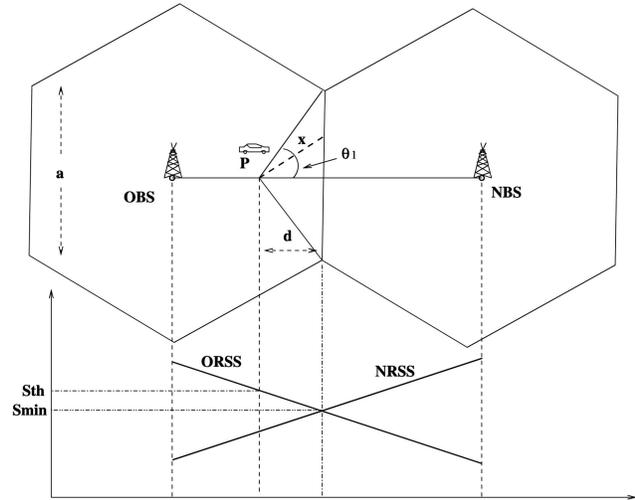
Fig. 2. Analysis of the handoff process.
