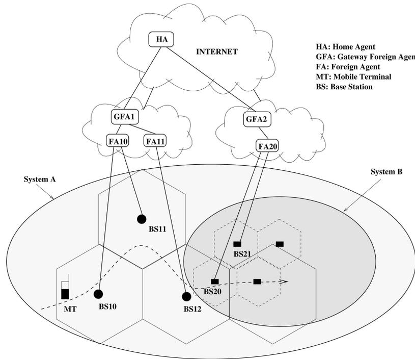
Fig. 1. Handoff in the integrated NGWS architecture.
