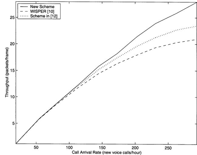
Fig. 8. System throughput (no CAC).
