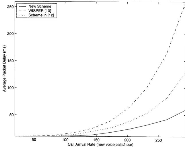
Fig. 6. Packet delay of remote login traffic (no CAC).
