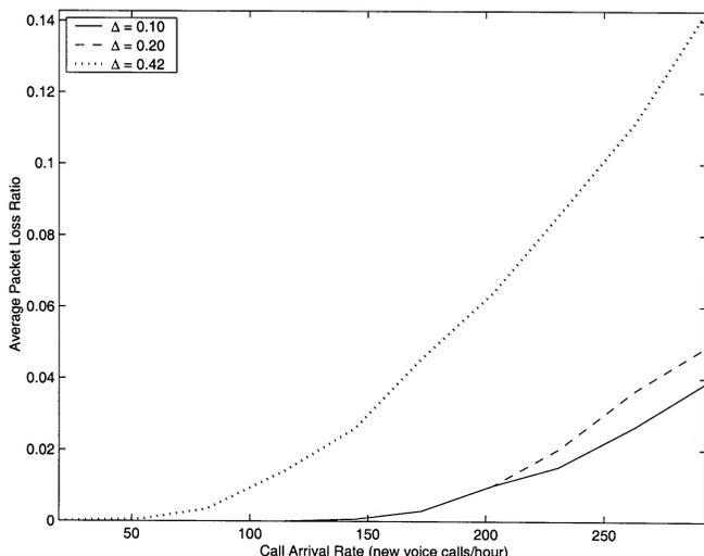
Fig. 11. Packet loss ratio of VBR video traffic.
