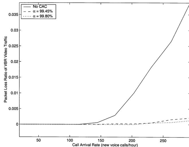
Fig. 15. Packet loss ratio of VBR video traffic (with CAC).
