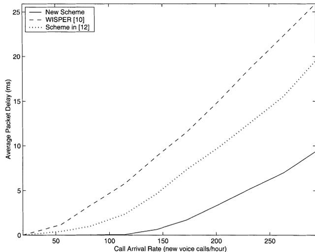
Fig. 5. Packet delay of VBR video traffic (no CAC).
