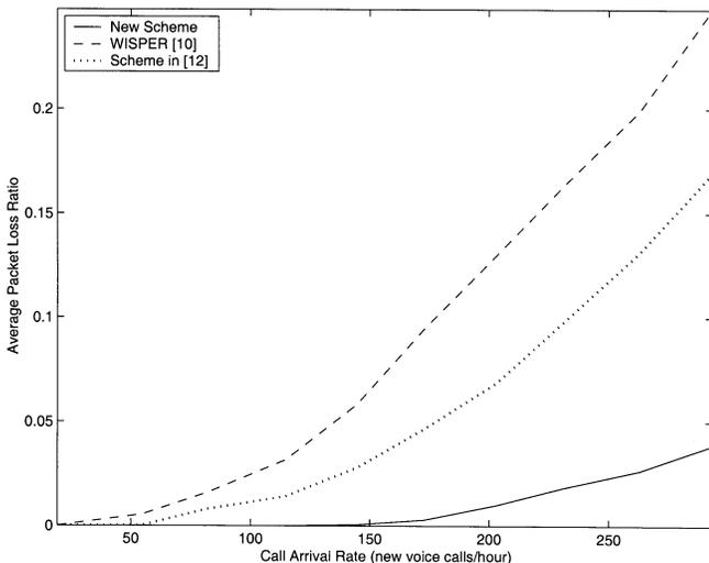
Fig. 7. Packet loss ratio of VBR video traffic (no CAC).
