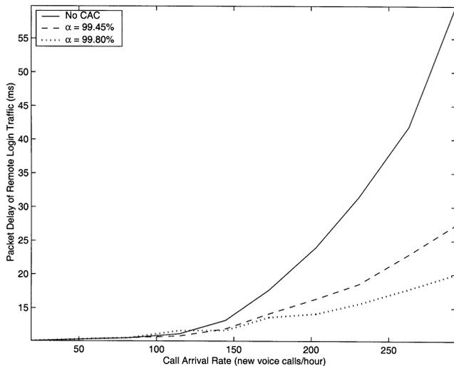
Fig. 14. Packet delay of remote login traffic (with CAC).
