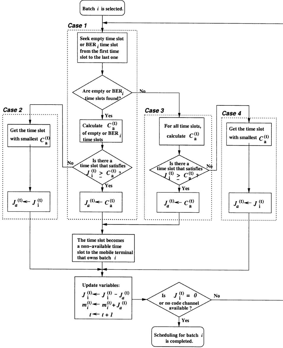
Fig. 4. Joint rate- and BER-scheduling scheme.
