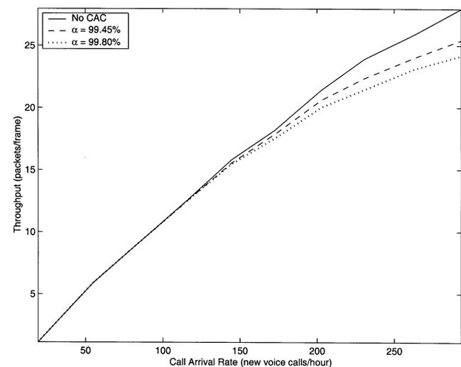
Fig. 17. System throughput (with CAC).
