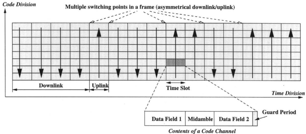
Fig. 1. The structure of one wide-band TD-CDMA frame.
