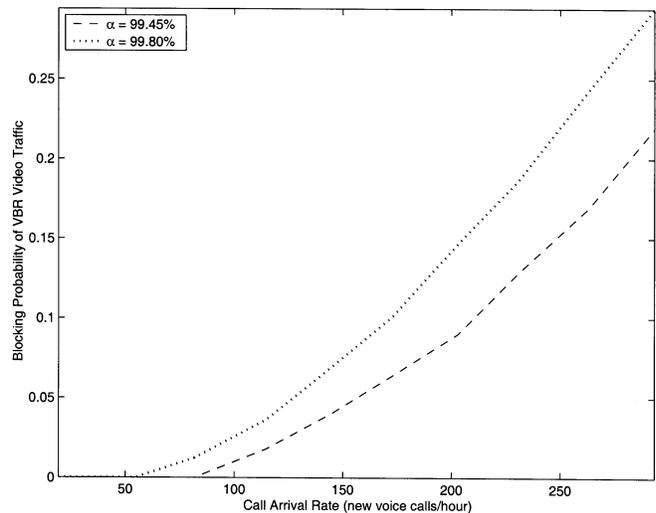
Fig. 16. Connection blocking probability.
