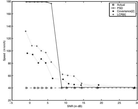
Fig. 4. Estimated velocity vs. SNR in Rayleigh fading environment for  $\tau = 1$  ms and  $T_{est} = 1$  s, and  $v = 40$  km/h.
