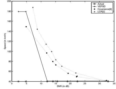
Fig. 6. Estimated velocity vs. SNR in Rayleigh fading environment:  $v = 40$  km/h, and  $T_{est} = 1$  s, and  $\tau = 0.5$  ms.
