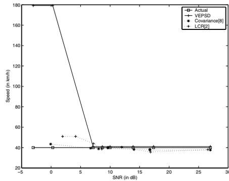
Fig. 5. Estimated velocity vs. SNR in Rayleigh fading environment:  $v = 40$  km/h, and  $T_{est} = 1$  s, and  $\tau = 2$  ms.
