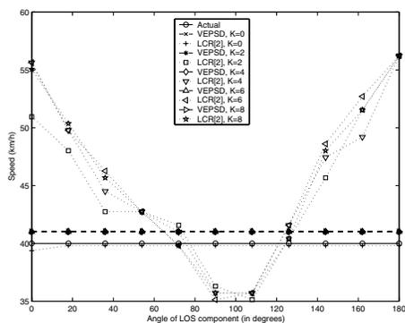
Fig. 9. Comparison of VEPSD estimator for  $v = 40$  km/h,  $\tau = 1$  ms,  $T_{est} = 1$  s, SNR=20 dB with LCR based estimator.
