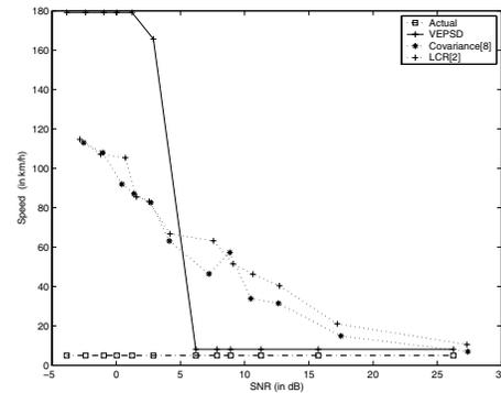
Fig. 3. Estimated velocity vs. SNR in Rayleigh fading environment for  $\tau = 1$  ms and  $T_{est} = 1$  s, and  $v = 5$  km/h.
