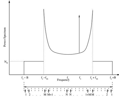
Fig. 1. PSD of received envelope in Rician fading environment in the presence of AWGN.
