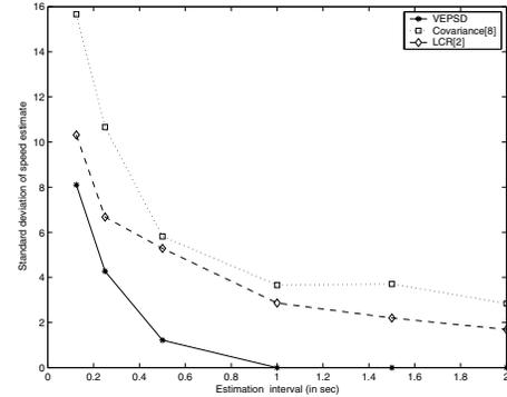
Fig. 2. Standard deviation of estimated velocity vs. estimation interval in Rayleigh fading environment:  $v = 40$  km/h,  $\tau = 1$  ms and SNR=20 dB.
