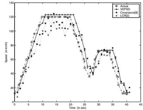
Fig. 8. Velocity tracking in Rayleigh fading environment:  $\tau = 1$  ms,  $T_{est} = 1$  s, SNR=20 dB.
