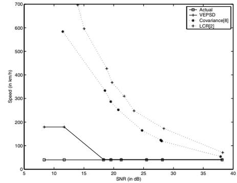
Fig. 7. Estimated velocity vs. SNR in Rayleigh fading environment:  $v = 40$  km/h,  $T_{est} = 1$  s, and  $\tau = 0.125$  ms.
