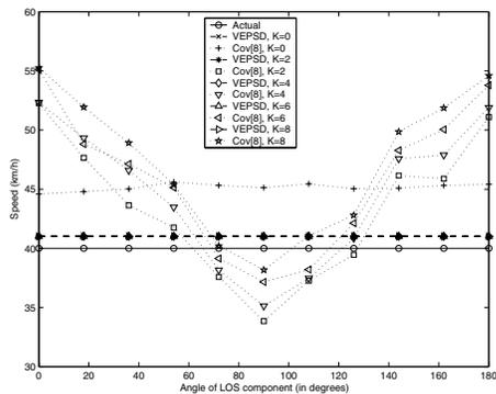
Fig. 10. Comparison of VEPSD estimator for  $v = 40$  km/h,  $\tau = 1$  ms,  $T_{est} = 1$  s, SNR=20 dB with co-variance based estimator.
