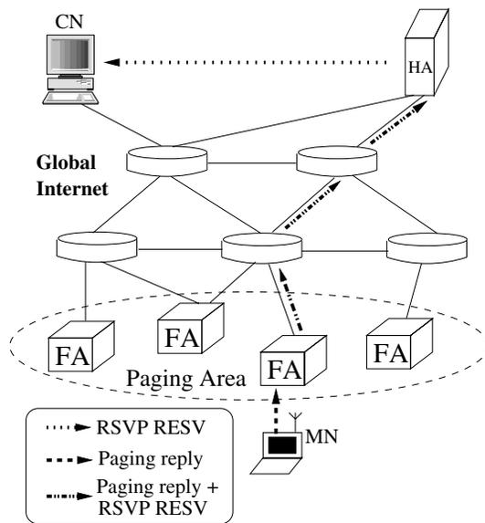
Fig. 4. Procedure of sending paging reply and RSVP RESV messages.
