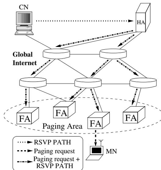
Fig. 3. Procedure of sending paging request and RSVP PATH messages.
