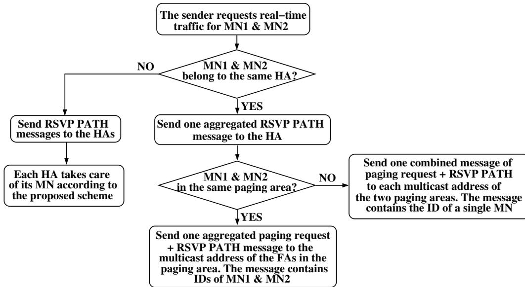
Fig. 5. Flow chart for multicast case.
