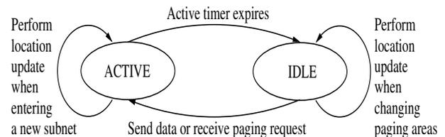
Fig. 1. State transition diagram of Mobile IP paging.
