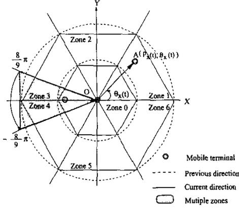
Fig. 3. Coordinate System with Zone Partition.
