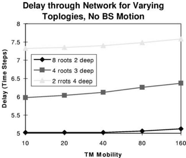
Figure 6. Delay through network as a function of network topology when the MBSs are fixed. MBSs at a particular level in the network were given a fixed amount of bandwidth.
