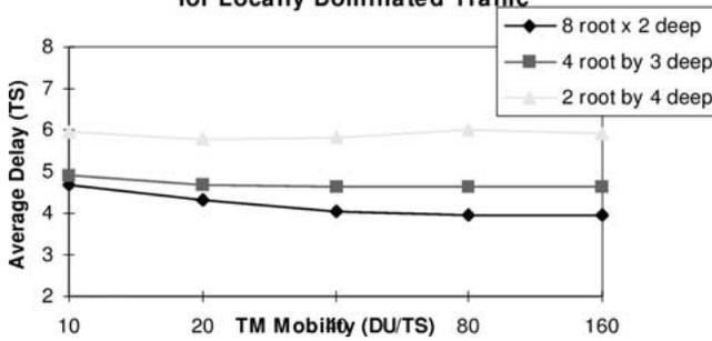
Figure 10. Average delay through the network for the case where the messaging is dominated by local traffic. For this plot, it was assumed that 60% of the traffic would remain within the tree of the sending MT.
