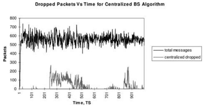
Figure 14. Lost packets versus time for the centralized load balancing algorithm. Conditions were the same as for figure 16 with the distributed algorithm.
