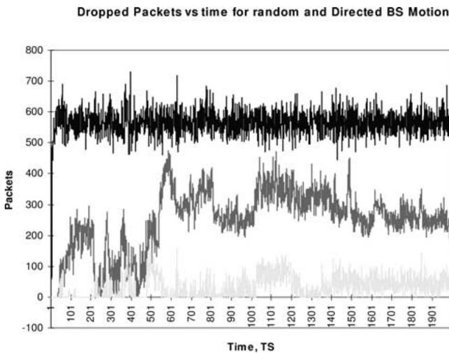
Figure 13. Dropped packets as a function of time for random MBS motion and directed MBS motion. Mobility rate was 80 DU/TS for MBSs and MTs. The top curve is the total packets offered to the network, the middle curve is the lost packet rate with no balancing, the bottom curve is the lost packet rate with the distributed balancing algorithm.
