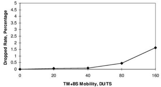
Figure 11. Dropped packet rate vs rate of motion of the MTs with no limit on network asymmetry, random motion of the MTs and MBSs.
