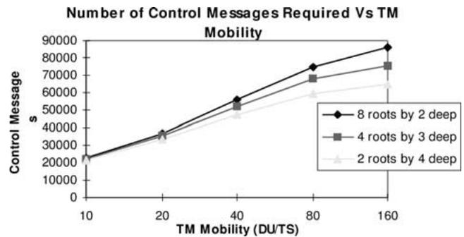
Figure 8. Number of control messages required as a function of the MT mobility. MBS mobility was fixed at a probability of 0.5 of moving 10 DU each time step.
