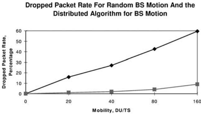
Figure 12. Comparison of the performance of the network for directed MT motion with no restrictions on network asymmetry with random MBS motion and a distributed algorithm to direct the MBS motion. The steeper curve is the case without load balancing.
