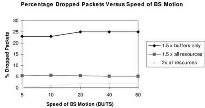
Figure 5. Dropped packet rate versus mobility of the MBSs (limited asymmetry in the network).
