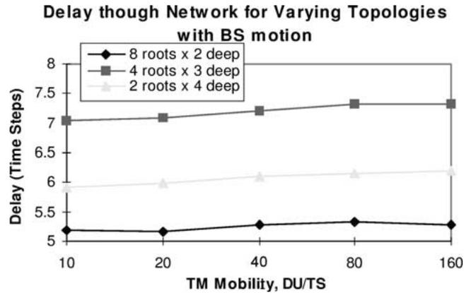
Figure 7. Delay through the network when the MBSs are allowed to move. The motion of the MBSs was set to have a probability of occurring during a time step of 0.5. When the MBSs do move, they move 10 distance units.
