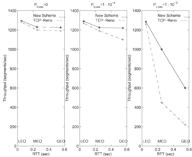
Figure 6. Performance comparison of TCP-Peach (solid lines) and TCP-Reno (dashed lines) when the SACK option is implemented for different values of loss probabilities.
