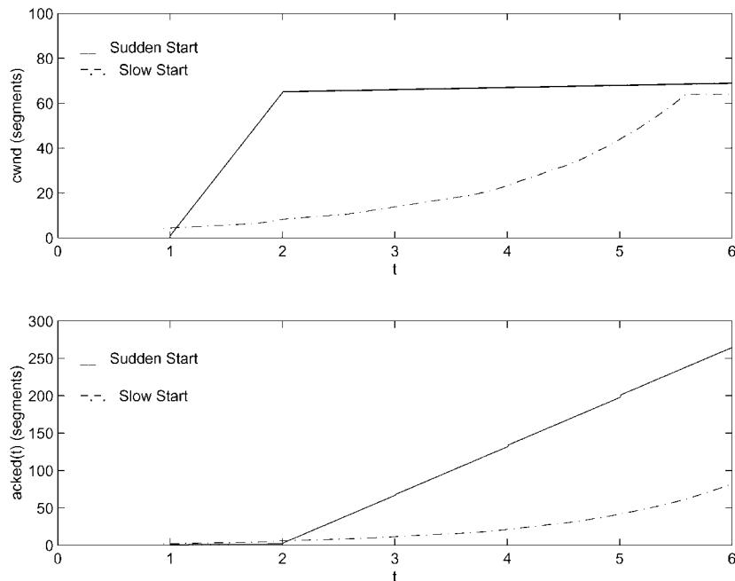
Figure 2. Comparison of the initial behaviour of TCP-Peach (solid lines) and TCP-Reno (dashed lines).
