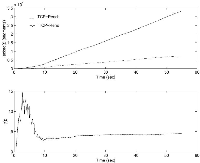
Figure 7. Behaviour of  $acked(t)$  for TCP-Reno and the TCP-Peach (upper plot) and of  $\gamma(t)$  (bottom plot).
