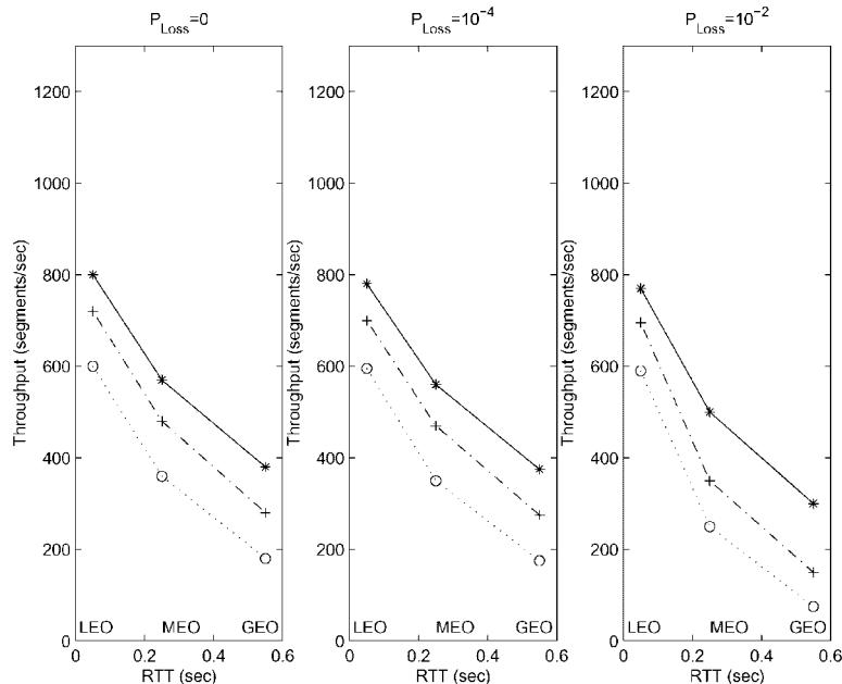
Figure 8. Transfers of files of  $S = 50$  segments: average throughput for TCP-Peach (solid lines), TCP-Reno (dotted lines) and TCP-Reno + IIW (dashed lines).
