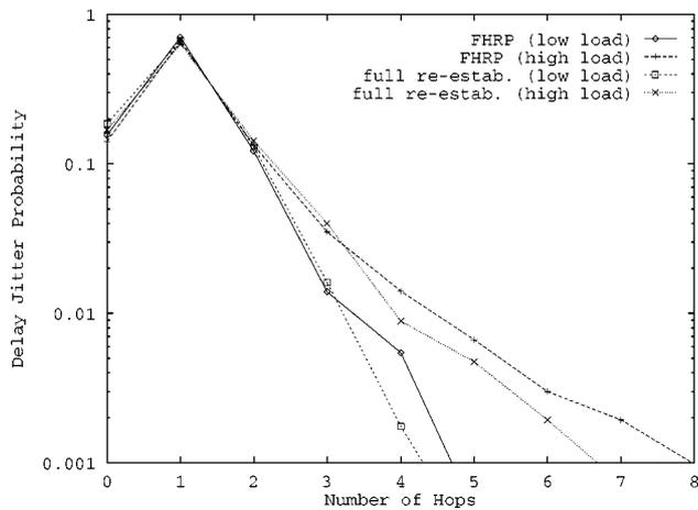
Figure 12. Probability density function of delay jitter for FHRP and full connection re-establishment.
