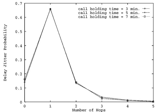
Figure 14. Probability density function of delay jitter for FHRP with different call holding times.
