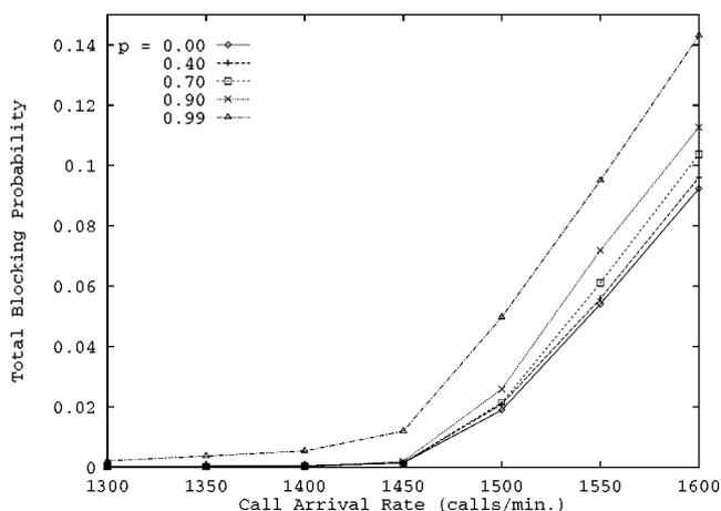
Figure 11. Total blocking probability as a function of call arrival rate and target probability.
