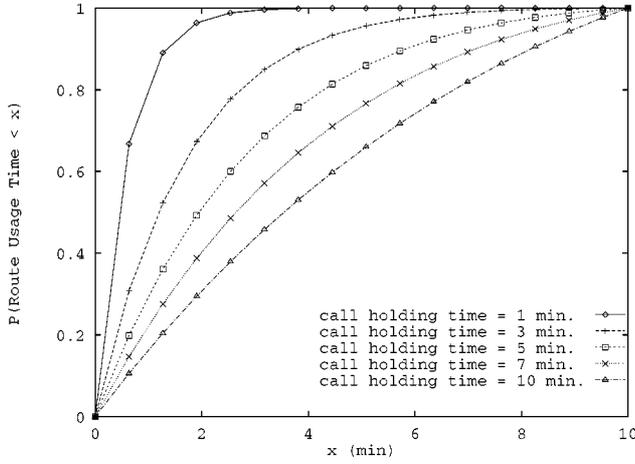
Figure 7. Route usage time pdf for various call holding times.
