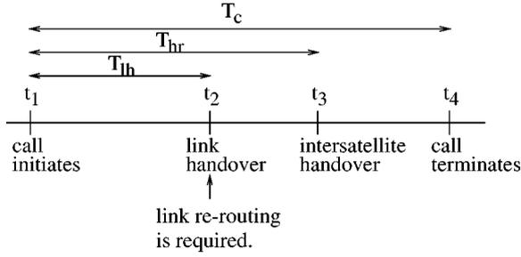
Figure 4. Timing diagram of call routing events.
