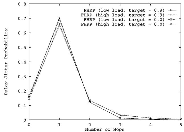
Figure 13. Probability density function of delay jitter for FHRP with target probabilities of 0.9 and 0.0.
