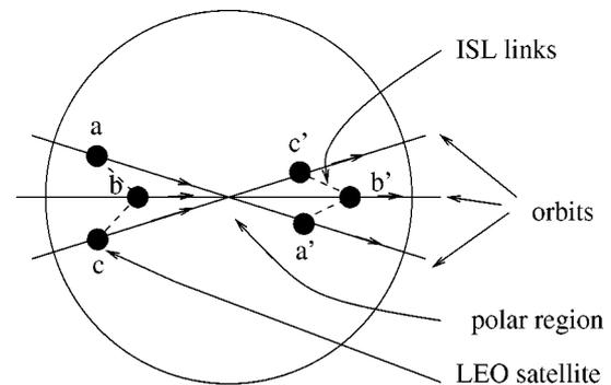
Figure 2. LEO satellites in polar region (top view).
