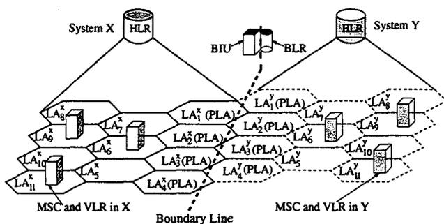
**Figure 1. An analytic model of two adjacent systems with boundary location register.**
