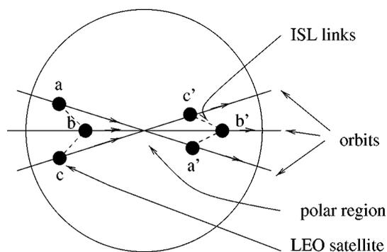
Figure 7. LEO satellites in polar region (top view).
