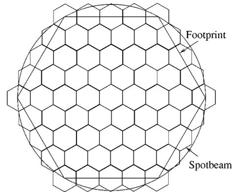
Figure 3. The spotbeams in a satellite footprint.
