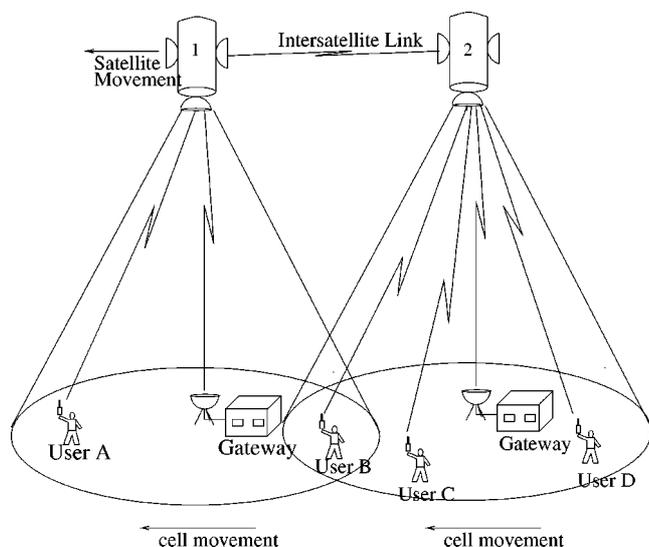
Figure 6. Wireless communication via Low Earth Orbit satellite network.
