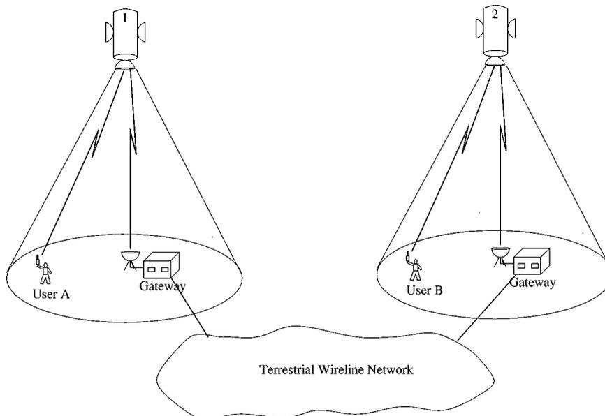
Figure 5. Low earth orbit satellite network with terrestrial routing.
