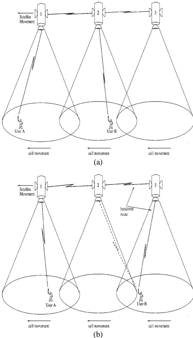
Figure 8. An intersatellite handover scenario: (a) The initial connection route between users A and B passes through satellite 1 and 2. (b) After user B hands over to satellite 3, the new connection route passes through satellites 1, 2, and 3.
