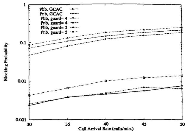
Fig. 5. The handover and new call blocking probabilities for slow spotbeams with nonuniform traffic distribution.
