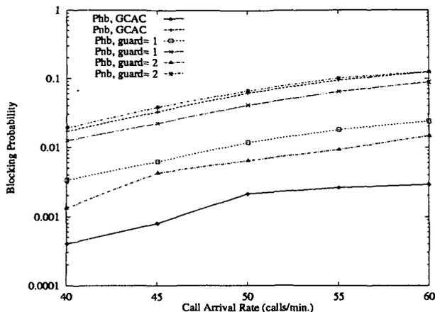
Fig. 3. The handover and new call blocking probabilities for slow spotbeams with uniform traffic distribution.
