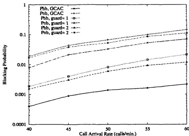
Fig. 4. The handover and new call blocking probabilities for fast spotbeams with uniform traffic distributions.
