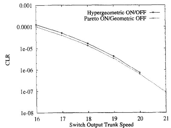
Fig. 9. CLR for two different arrival traffic models. The buffer size at the switches and the multiplexers is equal to 100 cells.
