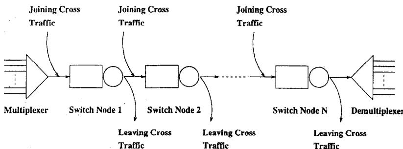
Fig. 1. Model of an ATM end-to-end connection.
