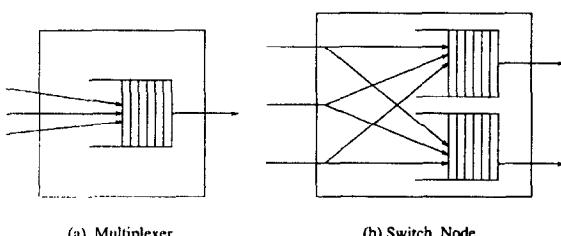
Fig. 2. Typical network elements: (a) a multiplexer and (b) a switch.
