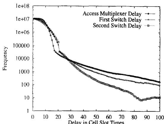
Fig. 10. Delay distribution frequency histogram at different hops of a connection. The buffer size at the switches and the multiplexers is equal to 100 cells. The multiplexer speed is 16 and the trunk speed is 20.
