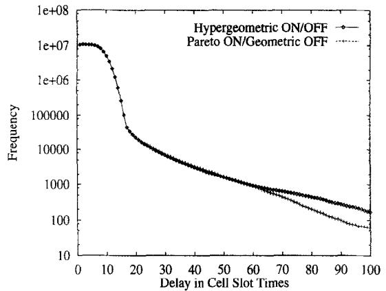
Fig. 11. Delay distribution frequency histogram for two different arrival traffic models. The buffer size at multiplexer is equal to 100 cells. The multiplexer speed is 16.
