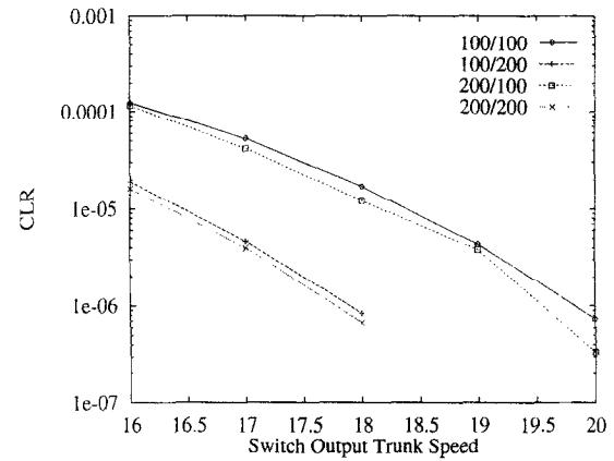
Fig. 8. CLR for different buffer size selection. In every configuration  $X/Y$  the  $X$  is the access multiplexer buffer size and  $Y$  is the interior switch element buffer size.
