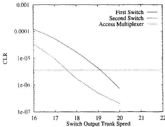
Fig. 7. CLR of the first and second switch for variable switch trunk speed versus the CLR at the access multiplexer. The buffer size is 100 cells at each multiplexer and each switch.
