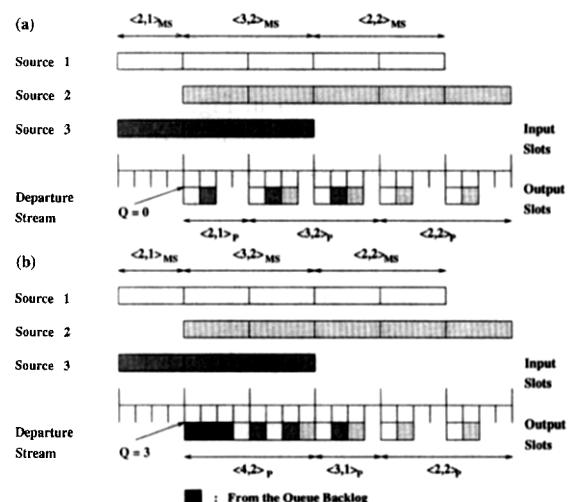
Fig. 4. Example of the departure process when  $C = 4$ , when (a) the initial queue length is zero, or when (b) the initial queue length is 3.
