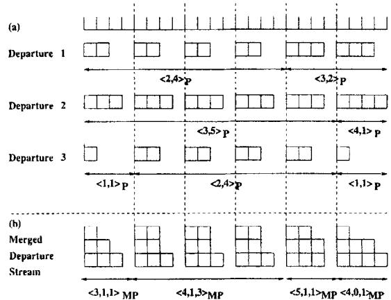
Fig. 5. Example of a departure stream merger when the link capacity,  $C$ , is 4.
