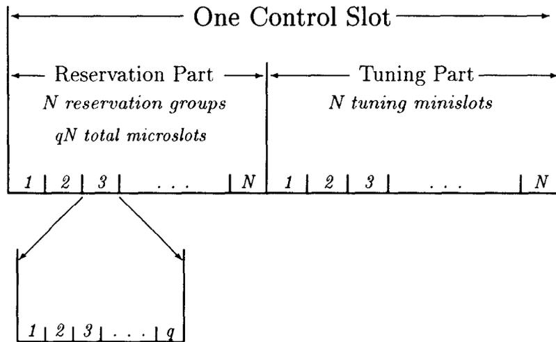
Fig. 1. Structure of a control slot.
