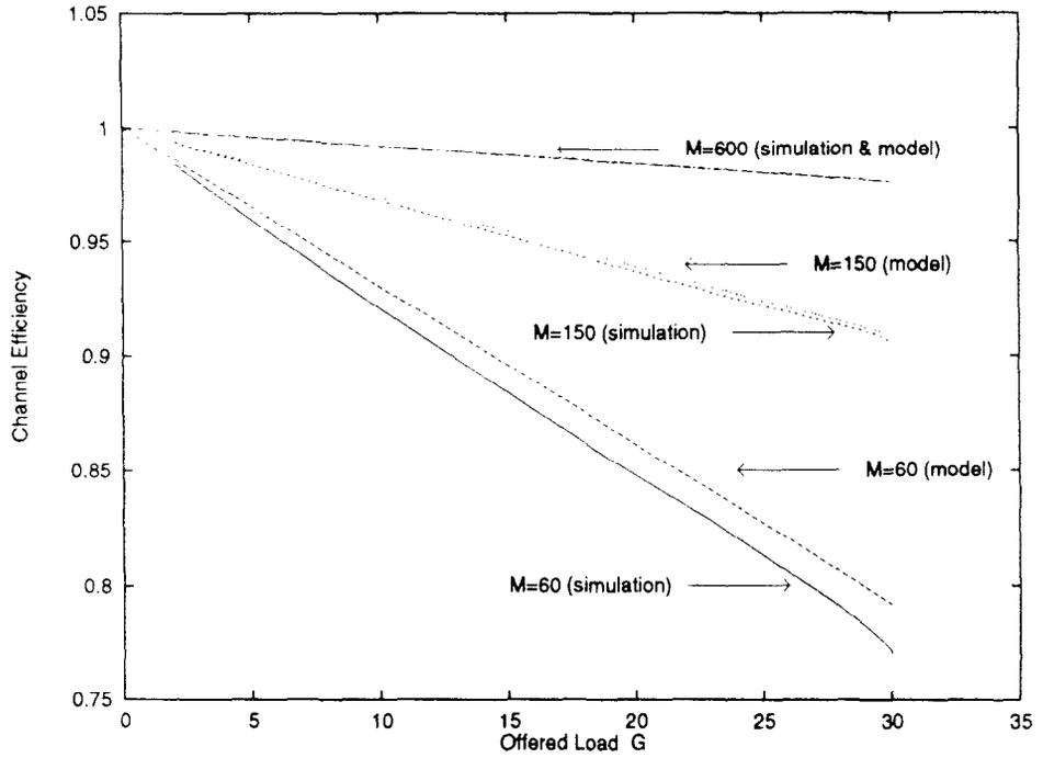
Fig. 8. Channel efficiency  $\eta_{NW}$  versus offered load, with  $N = 30$ .
