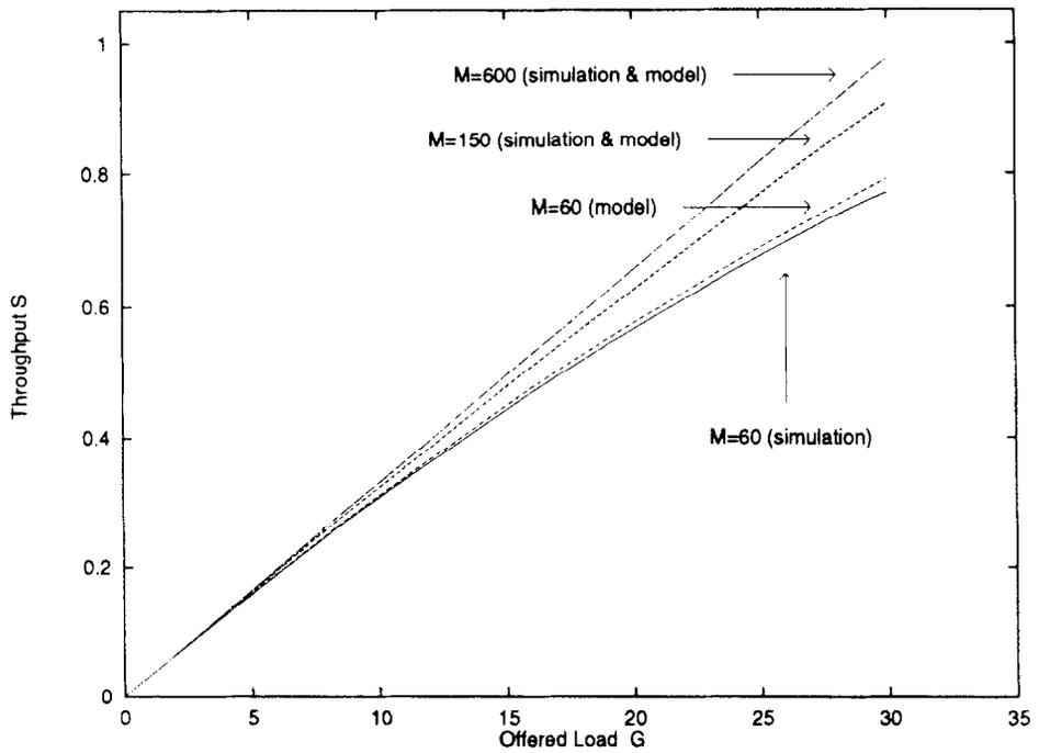
Fig. 6. Throughput  $S$  versus offered load  $G$ , with  $N = 30$ .
