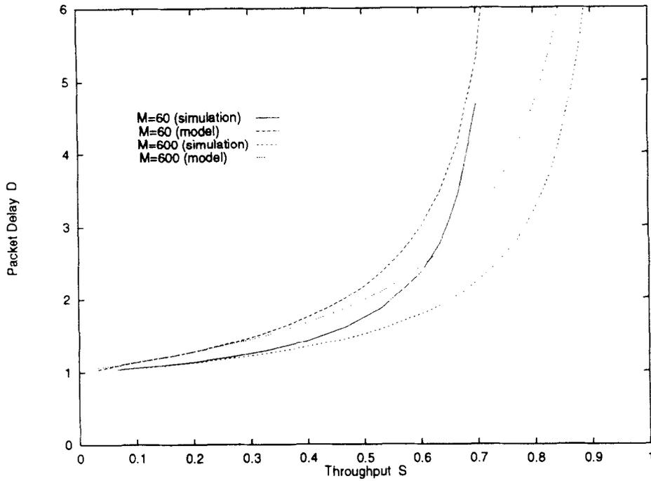
Fig. 10. Packet delay  $D$  versus throughput  $S$ , with  $N = 30$ .
