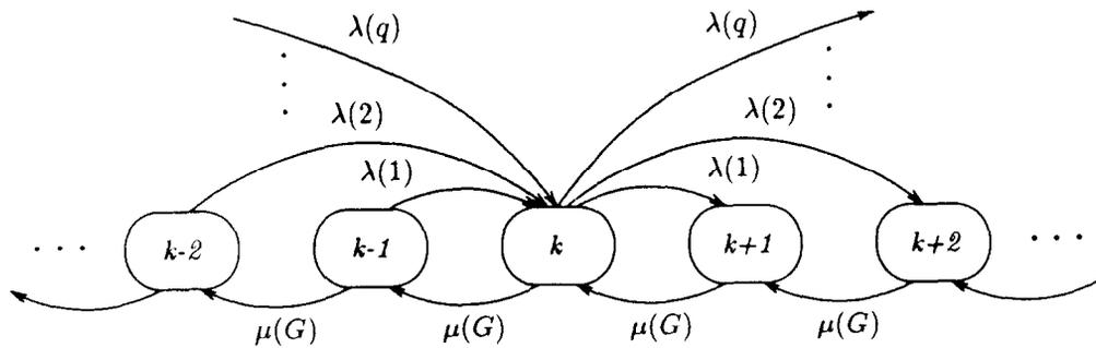
Fig. 4. The bulk arrival state-transition-rate diagram.<sup>1</sup>
