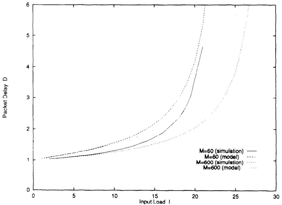
Fig. 9. Packet delay  $D$  versus input load  $I$ , with  $N = 30$ .
