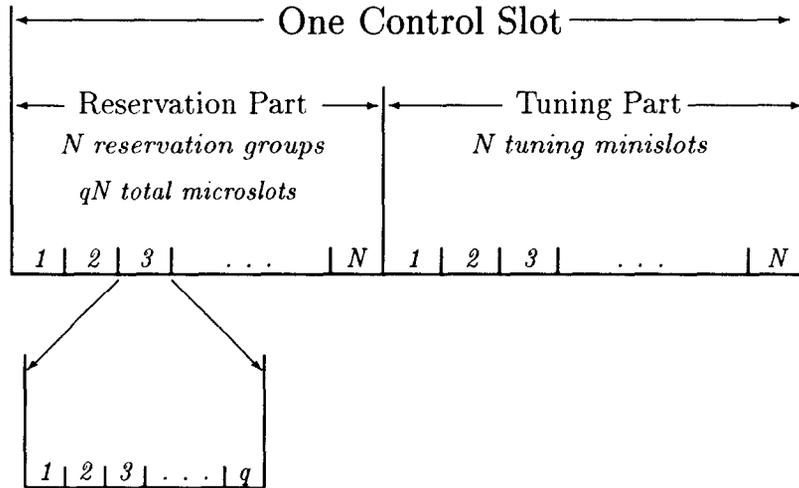
Fig. 1. Structure of a control slot.
