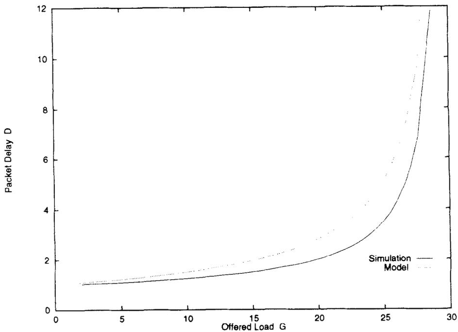
Fig. 11. Packet delay  $D$  versus offered load  $G$ , with  $N = 30$ .
