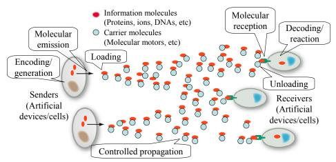
Figure 1. An example molecular communication system.
