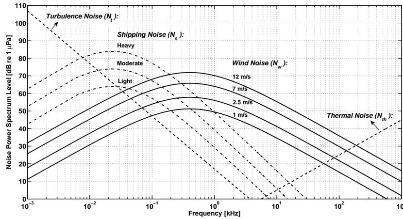
**Figure 23.4** The noise power spectrum level in dB re  $\mu$  Pa per Hz based on empirical formulae. Shipping noise is presented for *high* ( $s = 1$ ), *moderate* ( $s = 0.5$ ), *light* ( $s = 0$ ) shipping activities. Wind noise is shown for different wind speeds ( $w = 1, 2.5, 7$  and  $12$  m/s).
