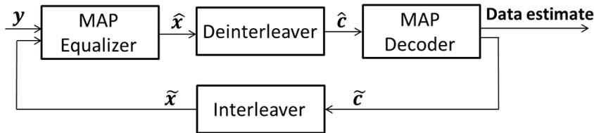
Figure 23.7 Receiver section with turbo equalization.
