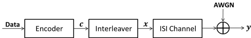
Figure 23.6 Transmission section of data transmitter system.
