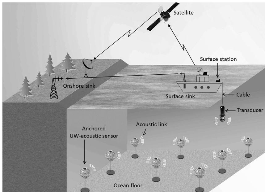
Figure 23.1 Architecture of an underwater acoustic sensor network.
