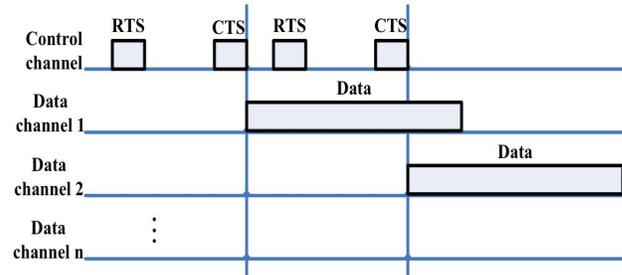
Fig. 7. Multiple Channels with Handshaking.
