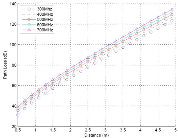
Fig.2 One-way path loss
