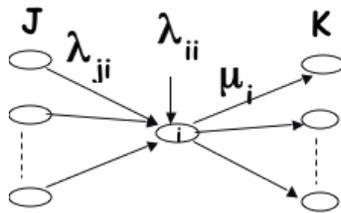
In this topology, node  $i$  has  $J$  upstream neighbors, from which it can receive relay packets, and  $K$  downstream neighbors, to which it can send its generated and relay packets. In this topology, the upstream neighbors  $(1, \dots, j, \dots, J)$  do not receive any relay packets and transmit only their generated packets.
