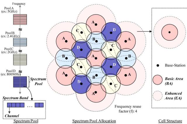
Fig. 1. Spectrum pool-based CR network architecture.
