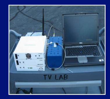
Prototypes designed to identify wireless microphone, NTSC and Digital TV signals
