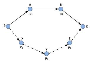
Whenever a channel switch occurs, there is switching time penalty of  $T_{sw}$ =1ms. The transmission time of a packet in the 600MHz and ISM band are  $T_{600}$ =3ms and  $T_{ISM}$ =5ms, respectively. Note that transmission is always first attempted on the licensed channel (i.e., the licensed channel is the default choice) at each node.
